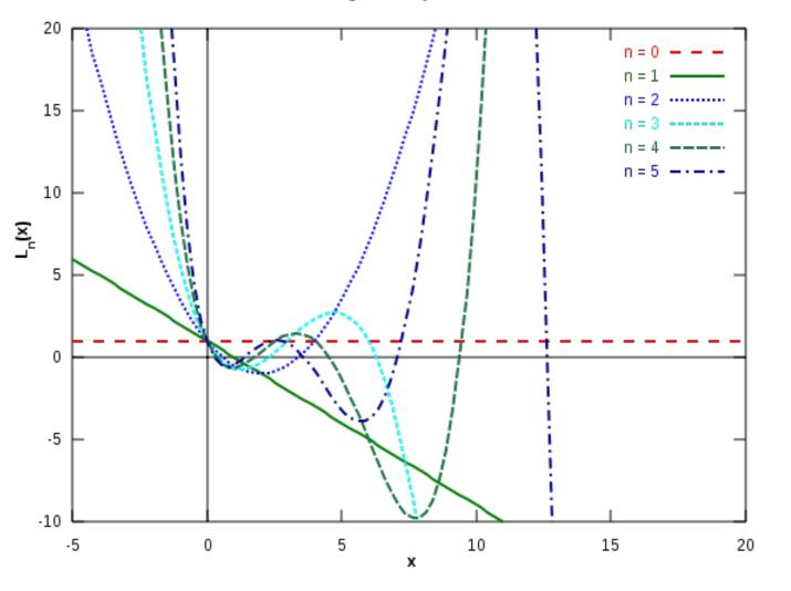
This figure shows a graph of the different Laguerre Polynomials with respect to different *n* values. You can see their corresponding roots/nodes which are,  $x_i$ : the i-th zeros of  $L_n(x)$ .
